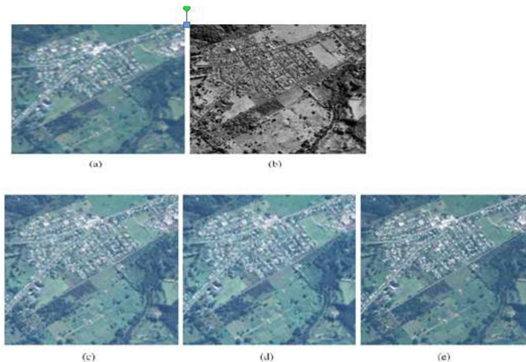
**Fig. 5.** QuickBird images and experimental results by the DNN-based pan-sharpening method. (a) LR multispectral image. (b) HR panchromatic image. (c) Fused image by the serial implementation of the DNN-based method. (d) Fused image by the proposed cloud computing framework. (e) Pseudocolor image of the reference multispectral image.
