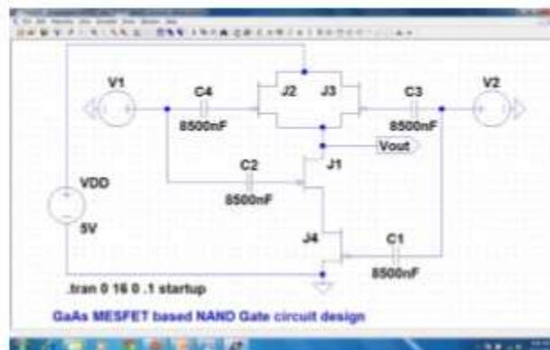
Fig. 2.1: GaAs MESFET based NAND Gate design circuit
